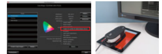
ColorNavigator 6.1 or above comes with a function to create an ICC profile for external devices
